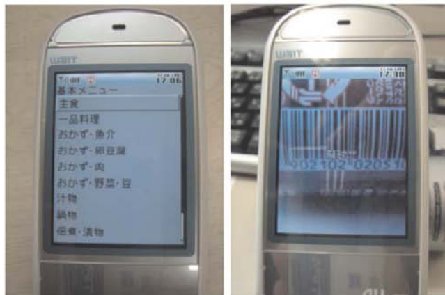
Fig. 3. Screen shot of menu selection method. Fig. 4. Screen shot of bar code input method.
