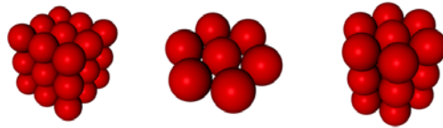
Figure 6: 3D cubic grid (left), 2D hexagonal grid (center), and 3D hexagonal grid (right)
