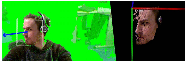
Fig. 1. Left: zoomed in original point cloud. The cube delimits a fixed size volume around the head. The blue arrow is an estimation of the pose. Right: the data within the cube are cropped, then rotated towards a frontal position and finally translated towards the origin.
