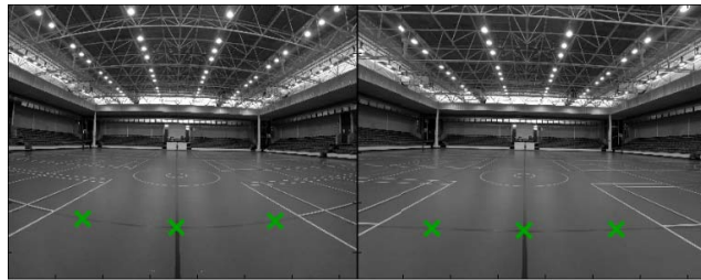
Fig. 4. Fisheye distortion before (left) and after (right) correction.
