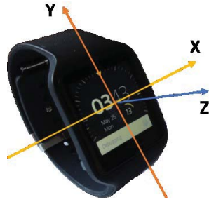
Figure 6: Sony Smartwatch 3 axis orientation
