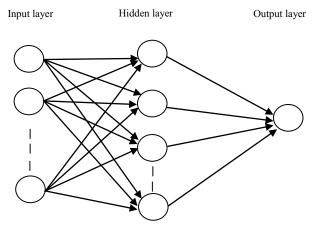
Fig 1. A simplified three layer neural network
