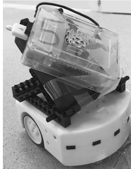
Figure 1: Thymio II robot, developed by The École Polytechnique Fédérale de Lausanne (EPFL) and École Cantonal d'Arts de Lausanne (ÉCAL), with Raspberry Pi B+, WiFi dongle, and external battery.
