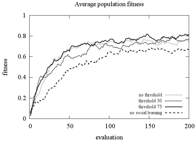
Figure 6: Lifetime learning without evolution in a group of 6 robots with identical sensory layouts. Time is measured by the number of evaluations ( x -axis), fitness by the formula in Section III ( y -axis) divided by the maximum fitness.
