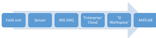
Figure 5. Methodology for data acquisition from the PD pump unit on site.
