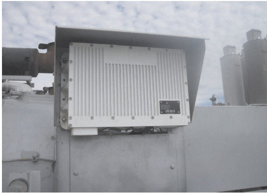
Figure 4. Data acquisition unit is installed in the field. Main characteristics are listed in the table.
