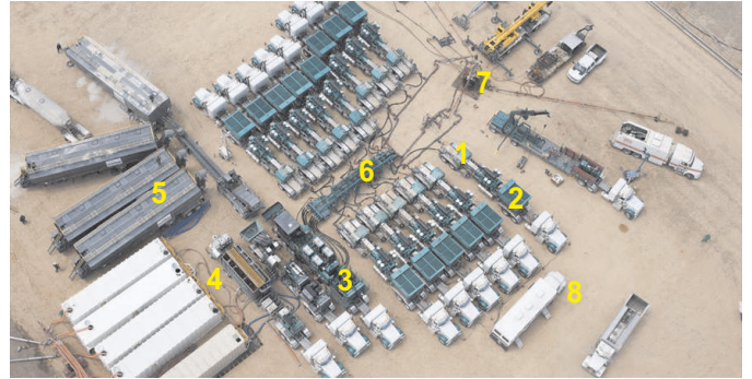
1 - PD pump 2 - Frac-truck assembly 3 - Blender - slurry mixer 4 - Water container 5 - Sand container 6 - Manifold trailer 7 - Wellhead 8 - Data collection van
