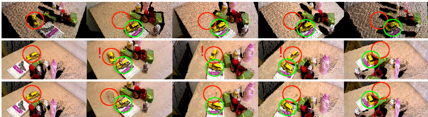
Fig. 6: Multiple observations of a scene observed in time from left to right with an object (yellow toy car) being moved twice within the sequence (top). Initial and new position of the object are marked red and green, respectively. The static environment assumed by the MVR [6] framework (middle row), incorrectly reconstructs the scene such that points from the object’s original position remain present during the whole observation period K (number of frames used) which was set to 3 in this experiment. Therefore, it took four observations for invalid points of the moved object to be discarded. Using our proposed change detection (bottom), the scene is correctly reconstructed at each time step. It removes points belonging to the old position of the object and keeps all points observed during the observation period that belong to the new object’s position or are static.
