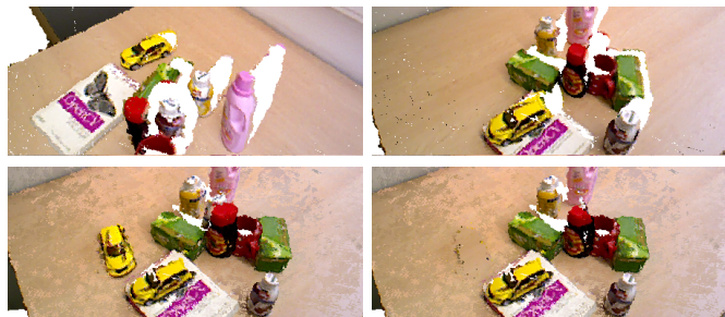
Fig. 1: Two views of a scene (top row) observed in time from left to right. In between the observations an object (yellow toy car) is moved in position. The bottom row shows the reconstructed 3D scene after the two observations, subsequently used as input for object recognition. In [6], the scene incorrectly contains two object instances of the yellow toy car in the reconstructed scene (bottom left). Using our proposed change detection module, only the instance in the current position is preserved (bottom right).
