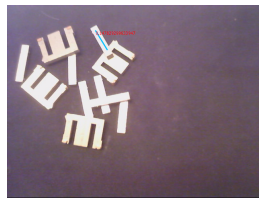
Fig. 10. Search of objects placed randomly with overlapping. Blue: Segment between the nodes. Red: Fitness function of the object.
