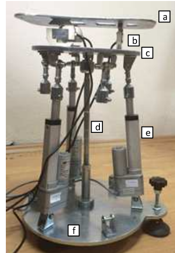
Fig. 1: The developed parallel ankle rehabilitation robot (a: Ankle connection platform; b: Force sensors; c: Moving platform; d: Central strut; e: Linear actuators; f: Base platform).
