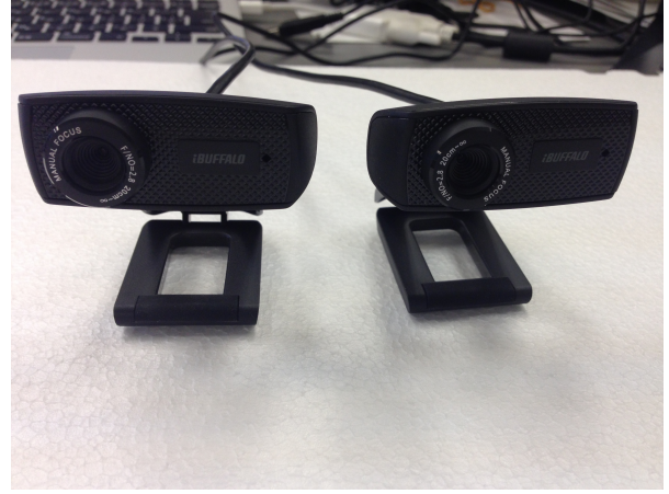
Fig. 7. Stereo cameras constructed by two web cameras
