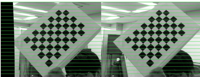
Fig. 5. Rectified left and right image by using checkerboard method
