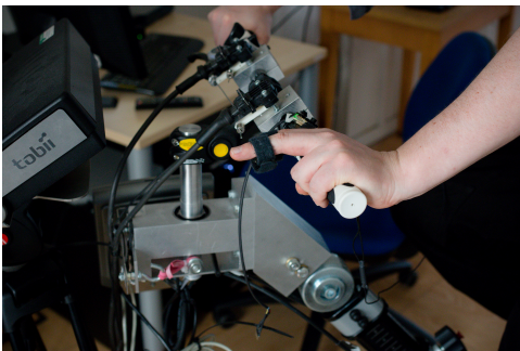
Fig. 3. Detailed View of the Experimental Setup: Rotatable Handlebar, Physiological Sensors connected to the Subject (EDA)
