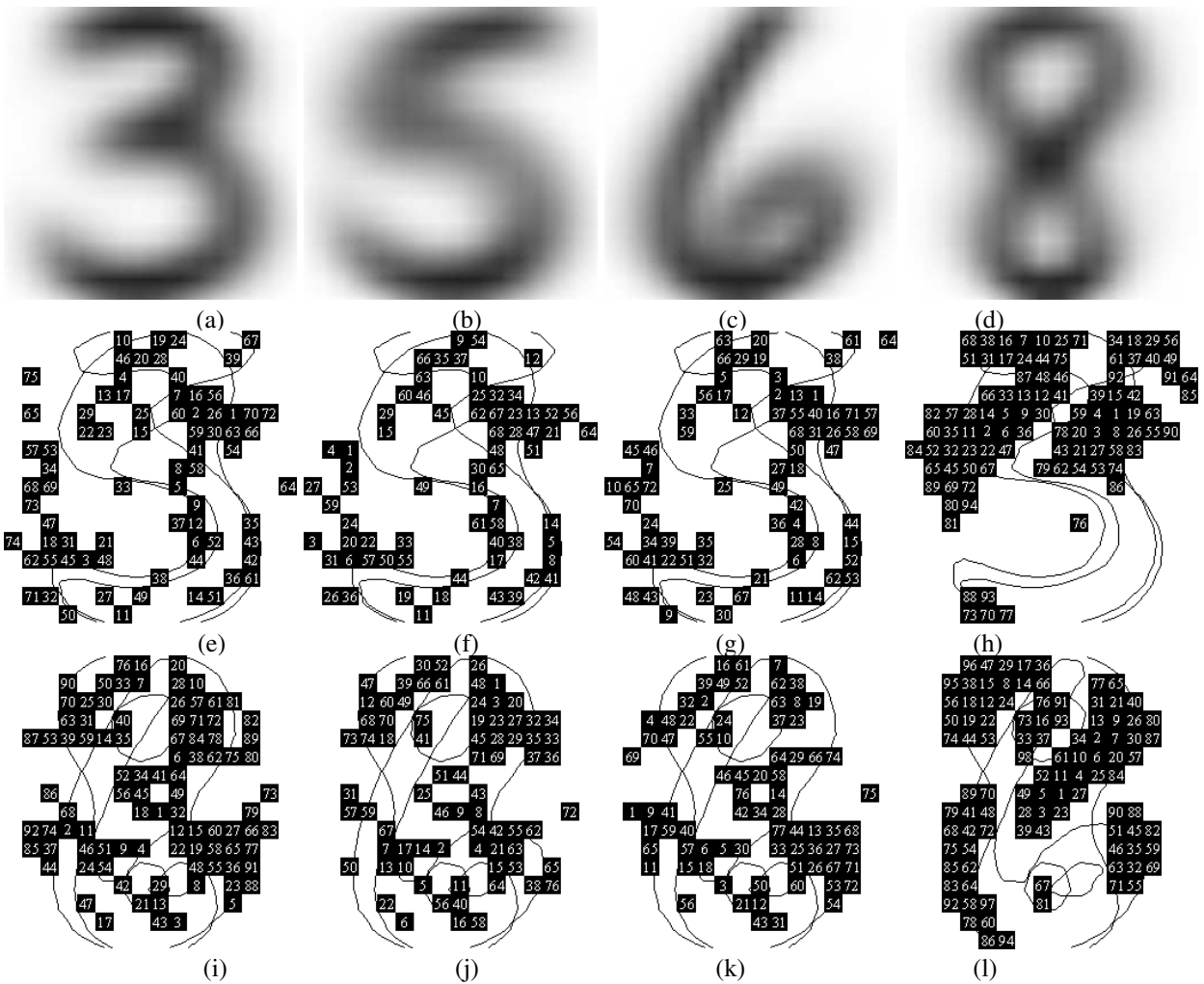
Fig. 3. Feature selection results for USPS subproblems. (a), (b), (c), (d) show the averaged digits, i.e. “3”, “5”, “6”, and “8”, respectively. From (e) to (h) and (i) to (l) are the results of SVM-RFE, SVM-SE, the combined method, and the baseline method. Blackened pixels are the selected features with the ranking order shown on each pixel.
