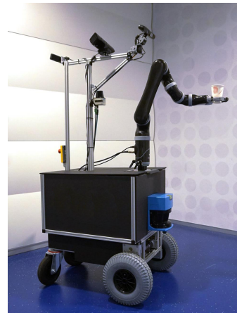
Fig. 6. The robot used for the experiments. The laser in the front of the robot is used for localization and obstacle avoidance. The two 3D sensors on both ends of the top bar are for 3D obstacle avoidance. The front sensor rotates based on the current speed of the robot to better detect obstacles.
