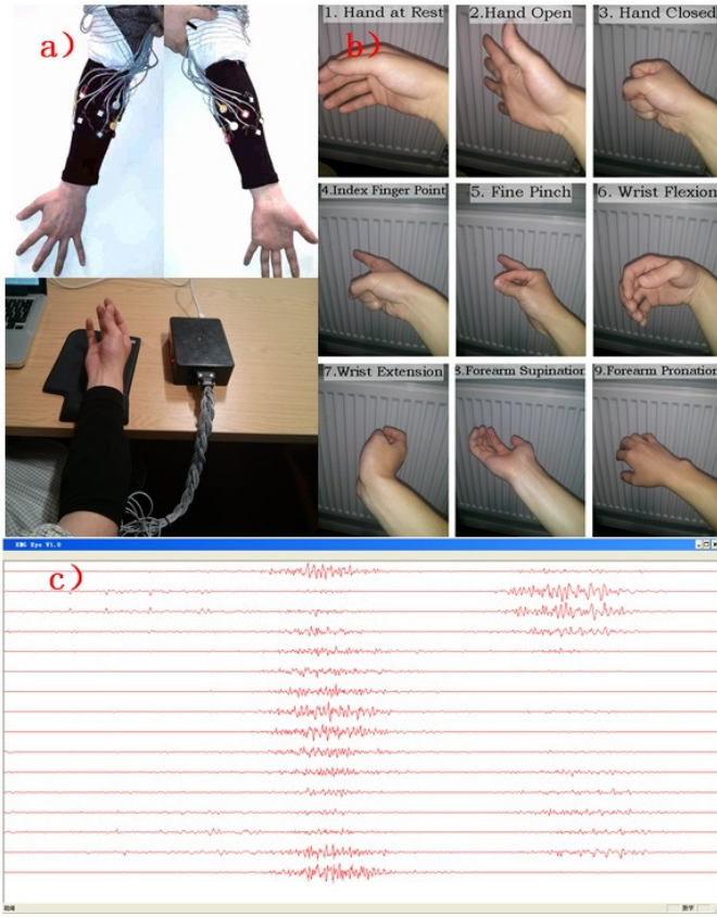
Fig. 4. From left to right, top to bottom: a. sEMG acquisition hardware including electrodes embedded sleeve and processing circuit b. 9 motions to be recognized c. display of 16 channels' sEMG samples [16]
