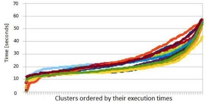
Fig. 2. Ordered times of the insertion task grouped by the construction of the product. Different colors show the different values of construction type attribute.
