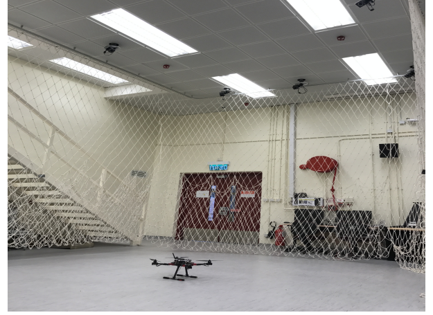
Fig. 4. The quadcopter equipped with PIXHAWK autopilot and vicon motion capture system
