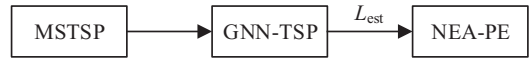
Fig. 2. The pipeline of the problem solving: the problem instance MSTSP, the prediction model GNN-TSP, and the problem solver NEA-PE.
