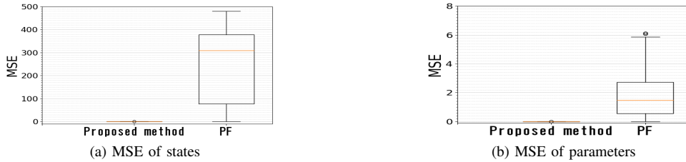
Fig. 3. The box plots of MSE values of the states and the parameters in the successful trials out of 100 trials of the proposed method and PF in the experiment using the Lorenz model. The smaller MSE is, the better performance is. The numbers of success trials of the proposed method and PF are both 100. The range between the bottom of the whisker and that of the box represents the best 25% trials. The range between the bottom of the box and the orange line represents the best 25% to 50% trials. The range between the orange line and the top of the box represents the best 50% to 75% trial. The range between the top of the box and the top of the whisker represents the best 75% to 100% trials. The points represent outliers.
