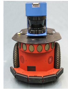
Fig. 4: Pioneer 3DX robot with a laser finder on top and 16 sonar sensors; 8 at front and 8 at rear.
