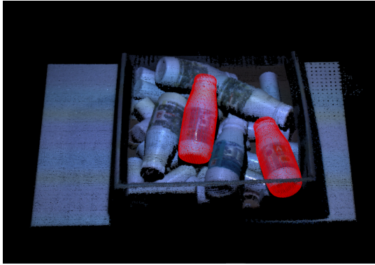
Fig. 6. The result of 6D object pose estimation with some bottles placed in a box with other objects. The two red objects are the output of 6D pose presented in a full 3D scene.
