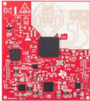
Fig. 1. TI IWR6843ISK-ODS board used for data collection.
