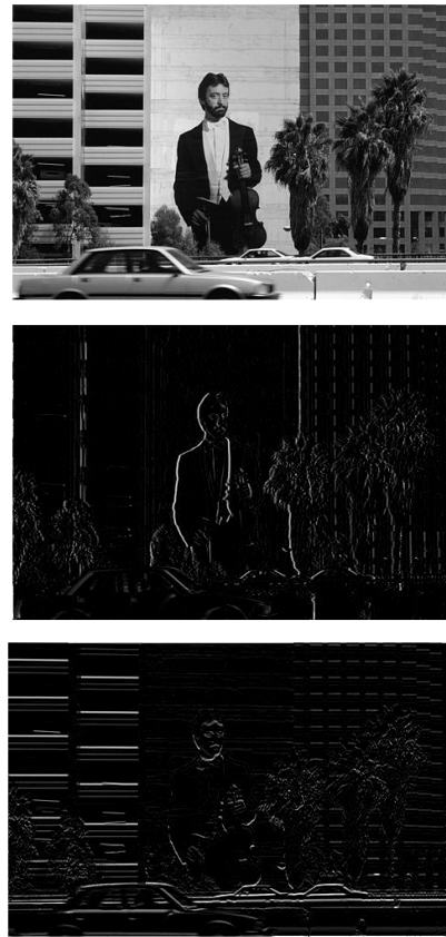
Fig. 3. Original, vertical and horizontal images after applying the Generalized Pre-Agregation \phi_v and \phi_h ( I_{119082}^{\phi_v} image from Berkeley dataset).
