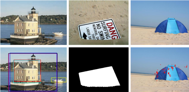
Fig. 2. Sample images from saliency detection and fixation prediction datasets [5][19]. Top row - input images, bottom row - different types of ground truth data, from left to right: human-annotated bounding box, human annotated pixelwise, eye-tracking results.
