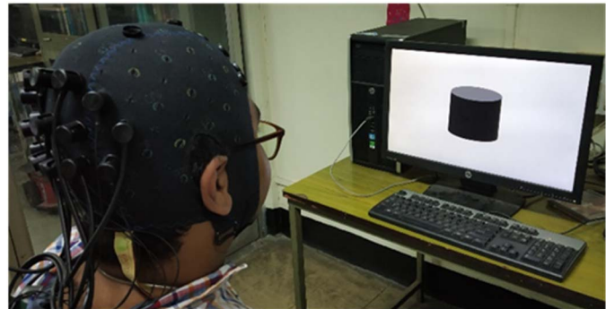
Fig.7. Capturing of parieto-occipital hemodynamic response during relative object size perception task performance.
