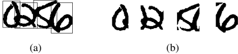
Figure 3. (a) Ground truth for a 4-digit string (0256) and (b) Shape of digits impacted by its neighbors.
