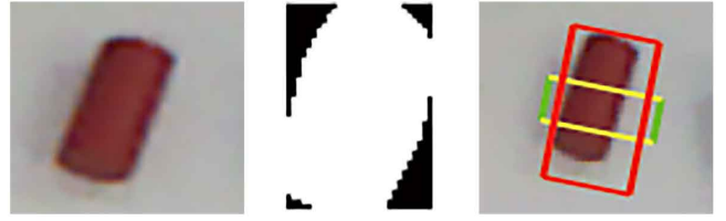
Fig. 2. A special case for our algorithm. From left to the right shows the original object, the convex hull of the object and the result of our algorithm. The red rectangle in the far right image is the bounding box for the red round rod and another rectangle is the generated grasp rectangle.
