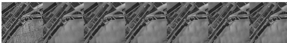
Fig. 5. Visual effect on the real SAR image. From left to right: SAR images, Lee, Kuan, SAR-CNN, ID-CNN and ours.
