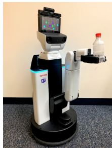
Fig. 2. The Toyota Human Support Robot [10], [11]. A scanning lidar at the base allows for SLAM mapping of the environment. A combination of height, arm, and gripper controls allows for objects to be picked up and put down on various surfaces. An RGBD camera allows for object segmentation, identification, and localization.
