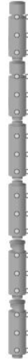
Fig. 1. A BCS system with six components and attached 36 sensors. Each square or circle represents a sensor.
