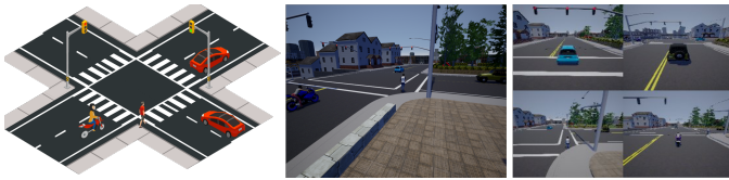
Fig. 1. Figure shows a heterogeneous multi-agent learning environment created using MACAD-Gym. An overview of the scenario is shown in the left image. The middle image shows the simulated scenario and the right image shows tethered views of each agent’s observation
