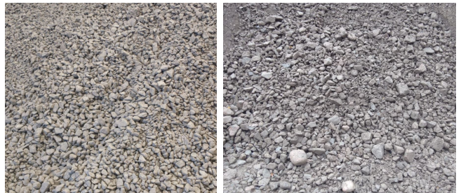
Fig. 5. Medium coarse gravel (left) and gravel-cobble material (right). Medium coarse gravel contains fine particles up to 64 mm, while gravel cobble material contains fine particles up to 200 mm.
