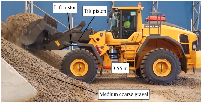
Fig. 1. Volvo L180H wheel-loader in manual operation.
