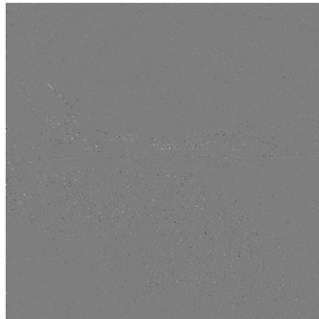
Fig. 9. The enhanced difference between the original image (Fig. 5) and the one filtered with MLMVN (Fig. 7) Image edges are well preserved.
