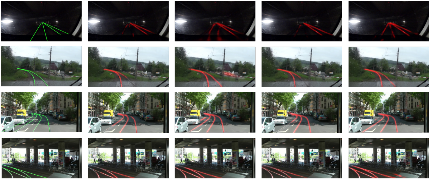
Fig. 4. Experimental results of several different algorithms on RailSem19 dataset. From left column to right column are the ground truth, VGG, SCNN, RailNet-LW, RailNet-AW results.
