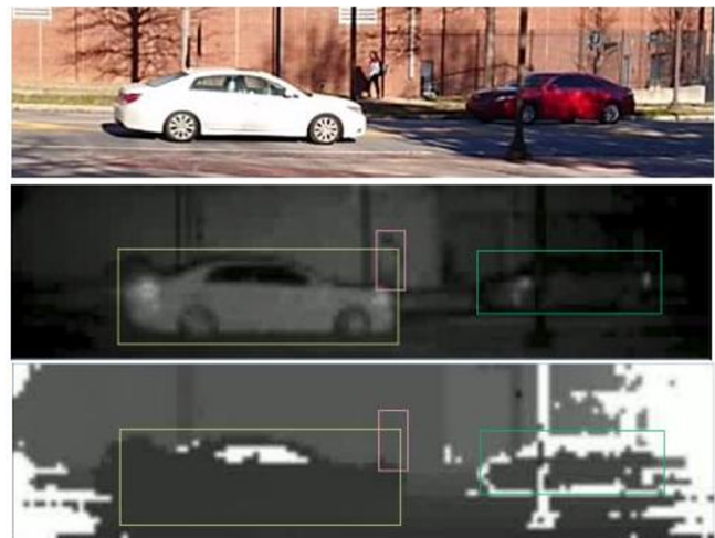
Fig. 1. Sample Image from extended CAMEL dataset. RGB Image(Top) has been cropped to cover area of intersection between FoVs of RGB camera and flash Lidar. Flash lidar Image with intensity channel is shown in middle row and depth channel in bottom row. Subjects of interest such as car, van and person are annotated in flash lidar image.
