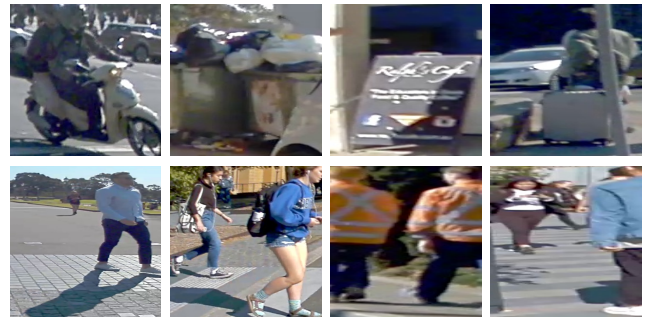
Figure 4: The top row depicts samples rejected as pedestrian by the 3D CNN. The bottom row shows samples incorrectly confirmed as pedestrians. Note that all these samples were detected as pedestrians by the 2D object detectors.
