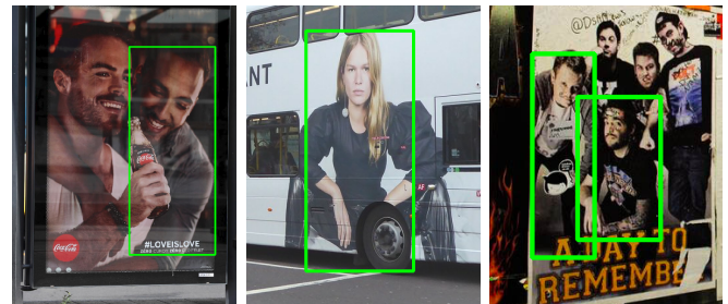
Figure 1: Output of a state-of-the-art object detector. The detections are not correct in a self-driving cars context because they are not actual persons, but depictions of them.
