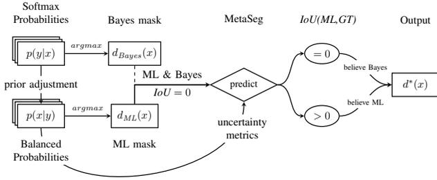
Fig. 1. Overview of our method for controlled false negative reduction of minority classes which we term “MetaFusion”. Note that  $IoU$  denotes the intersection over union measure of two segmentation masks.
