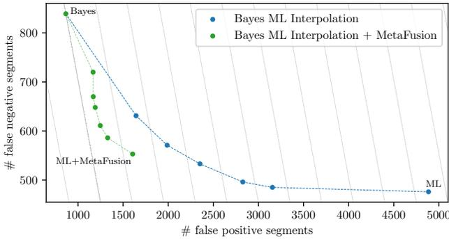
Fig. 3. False positives vs. false negatives of human segments for MobileNetV2 on Cityscapes. The blue curve is obtained by applying adjusted decision rules according to equation (16) with varied degrees of prior interpolation  $\alpha$ . For each of the points given on the blue curve we additionally apply MetaFusion which results in the green points given in the figure. The diagonal gray lines depict level sets along which the sum of both errors is constant.
