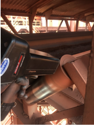
(b) Ultrasound recording of a conveyor idler in the MTPM.
