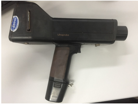
(a) Ultrasonic sensor Ultraprobe 10000 (UE Systems Inc.)..
