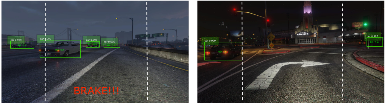
Fig. 2: Brake command generation. The area within the white dotted lines illuminates the trajectory of the self-driving agent. The left image includes a vehicular object which is within the driving trajectory of the self-driving agent and at an unsafe distance, so our model issues a brake command to stop our self-driving agent; the right image shows a vehicular object which is not at a safe distance but not within the driving trajectory of our self-driving agent, so our model issues no brake at this moment.
