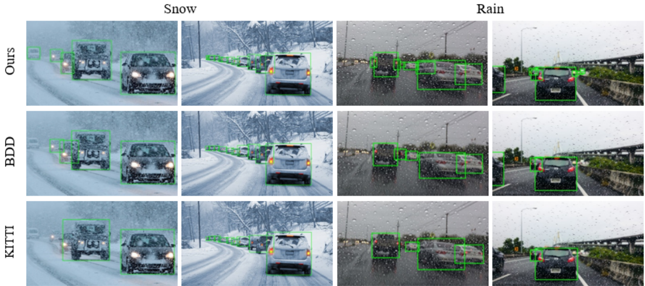
Fig. 6: Demonstration of detection results from networks trained by ours, KITTI and BDD dataset. We use examples from R-FCN. The top row demonstrates examples from a network trained by our simulation dataset; the middle row demonstrates examples from a network trained by KITTI; and the last row demonstrates examples from a network trained by BDD.
