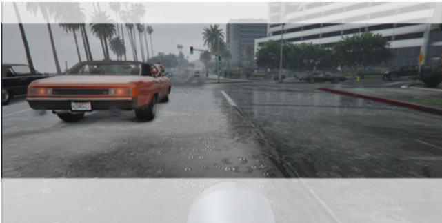
Fig. 3: Image pre-processing. The sky and headlight of the scooter are removed.
