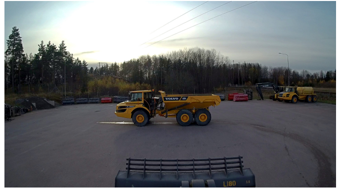
Fig. 2: Example of an image from the full-scale test data with a wheel loader that approaches the dump truck from the side.
