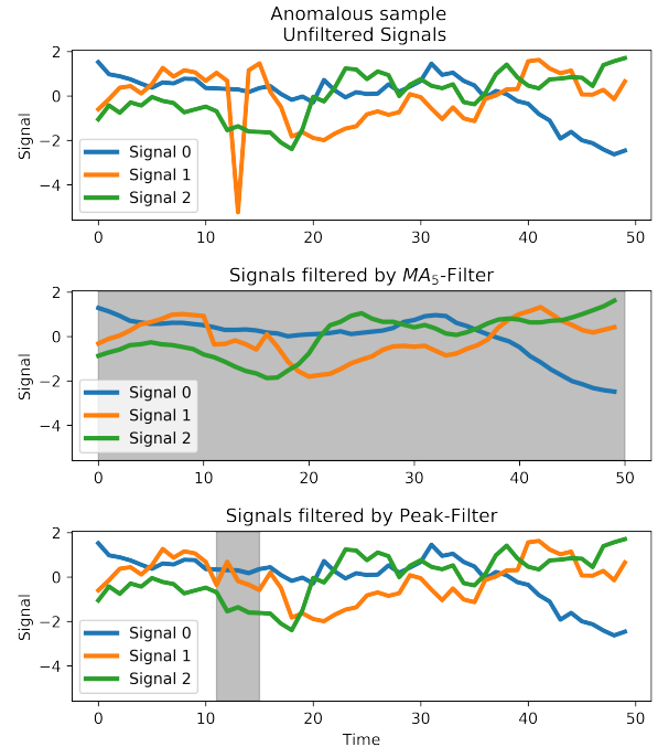
Fig. 8. Applying the MA_5 -filter flips the prediction for the anomalous sample, but affects the full time series. The MaskPeak-filter has almost the same effect on the network prediction, but modifies only few data points. Here, it affects the peak of Signal 1. (Modified data areas are marked gray.)
