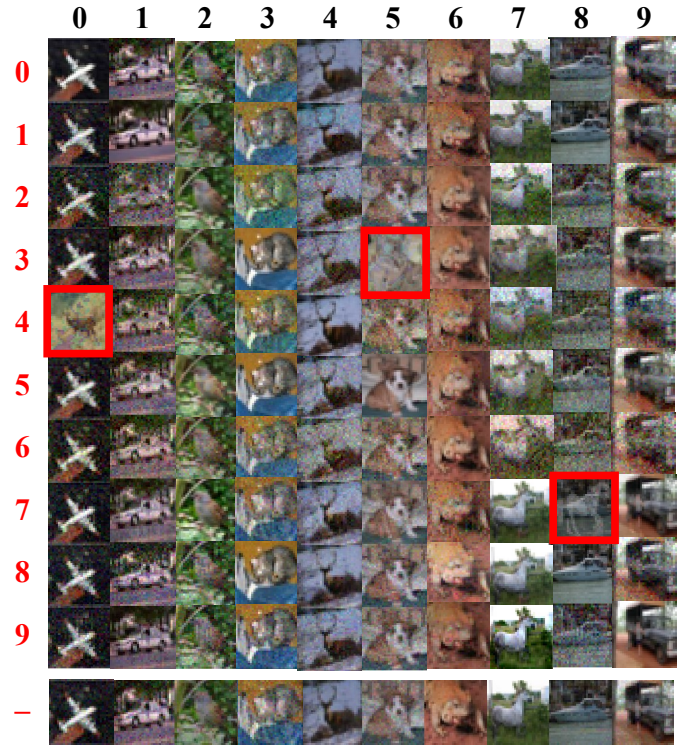
Fig. 6: Performing the Targeted and Un-targeted Attacks on the classifier using only the decision provided by the classifier. (Top 10 rows) Adversarial examples found for the targeted attacks. Correct labels are shown top in black on top. The target labels are shown in red on left. (Last Row) Adversarial examples found for un-targeted attacks. Maximum number of queries = 10^5
