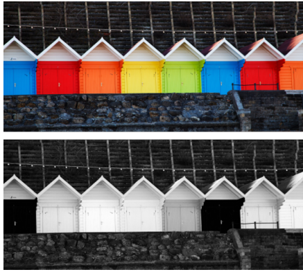
Fig. 2. Top: An RGB image viewed without the spectral filter. Bottom: The image viewed through a red spectral filter. The filter attenuates the Green channel and blocks the Blue channel. Pixels with high red content are perceived past the filter as bright, while pixels with low Red content are seen as dark. (Best viewed in color).
