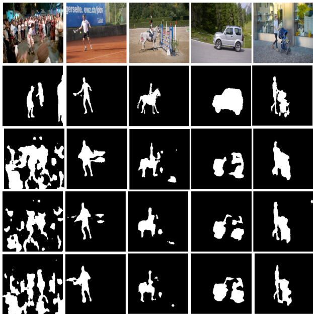
Fig. 9. Visual outputs of testing our network variations for video object segmentation on DAVIS dataset; Row 1: Input image, Row 2: Segmentation groundtruth; Row 3: ResNet-STLSTM output, Row 4: I3D-ResNet output, Row 5: I3D-STLSTM-ResNet output
