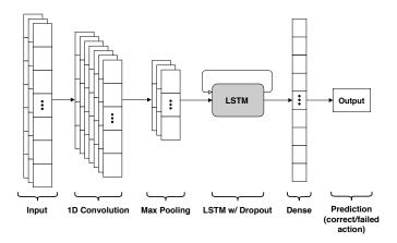
Fig. 3. LSTM network architecture: the input layer is followed by a 1D convolution layer (with 100 filters of size 20 and ReLU activation function), max pooling operation (with a pool size of 2), LSTM block (with 100 cells), dropout layer (with rate 0.5) and finally a dense layer with the sigmoid activation function.
