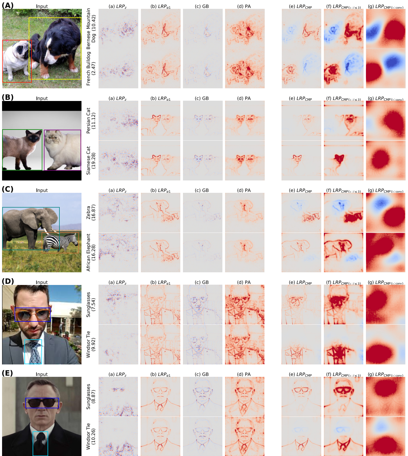
Fig. 4. Different attributions for the output classes “Bernese Mountain Dog” and “French Bulldog” (A), “Persian Cat” and “Siamese Cat” (B), “Zebra” and “African Elephant” (C) and “Sunglasses” and “Windsor Tie” (D and E), using the pretrained VGG-16 model. For details cf. Fig. 1.
