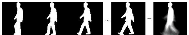
Fig. 2. Silhouettes extracted from a gait cycle, where the rightmost correspond to the Gait energy image.
