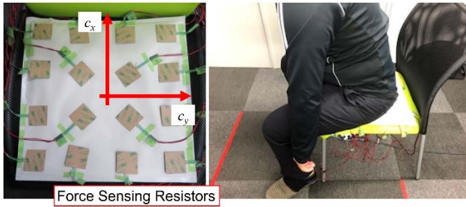
Fig. 3. Mattress pressure sensor with 16 force sensing resistors for measuring user's center of gravity to control the mobile robot.
