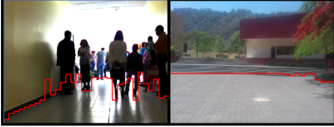
Fig. 5. Generalization capacity of StixelNet using two validation images, detected obstacles are drawn with red lines for every 20 horizontal pixels.
